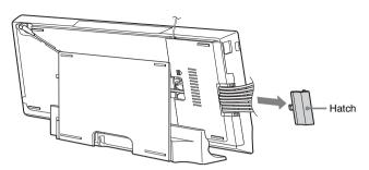
To open the hatch, remove the panel cover, hold the hatch, and then pull it up and outward. To close the hatch, align the projection of the hatch with the projection opening on the panel cover, and then gently push in and down on the hatch until it clicks.
